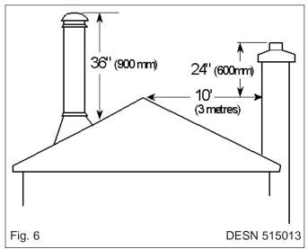
Illustration showing minimum heights required, depending on the location of the chimney.
